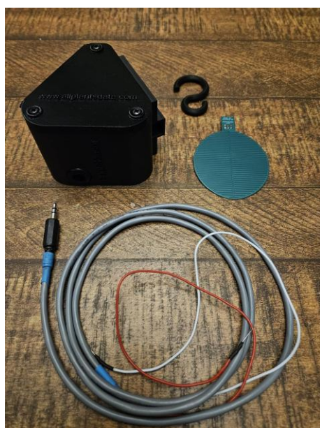
Tag, hanger, electrode cable and leaf-wetness sensor
