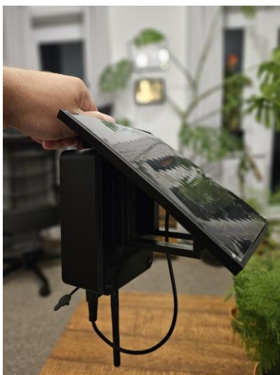
Panel mounted on the gateway
